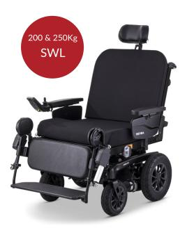
This Meyra XXL Electric Wheelchair won't let you down. It's built to move users up to 250kg, with a great stable and sturdy design, the XXL is tough. Thanks to the power tilt-inspace function, as well as the choice of powered separate swingaway powered or manual footrests, you can be more comfortable.
